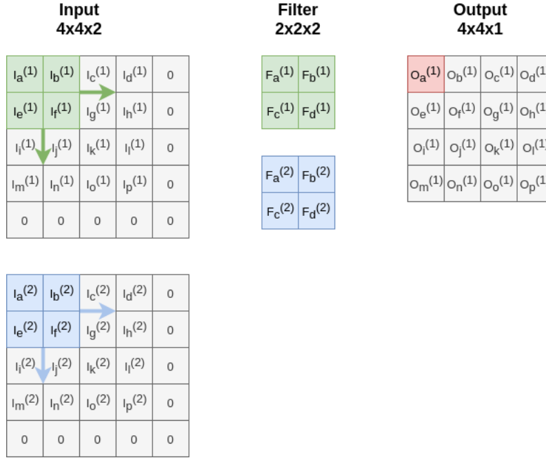
Figure 2.2.: In this figure, we illustrate the application of convolution on a 3-dimensional input with a single 2 \times 2 filter, and a stride of 1, represented by the horizontal and vertical arrow. Thus, the output is computed by the dot product of the receptive field of the input and the filter. More precisely, the output at position O_a^{(1)} represents the sum of 1) the dot product of the receptive field of the first input layer (green), and the corresponding filter (green), and 2) the dot product of the receptive field of the second layer (blue) with the corresponding filter (blue). The remaining output fields are computed in the same way, while sliding one step at a time over the input. [Goodfellow2016, Karpathy2019] Additionally, to preserve the input dimension for the output, we introduce a zero-padding to the input. [ https://www.youtube.com/watch?v=qSTv_m-KFk0&feature=youtu.be (Accessed on: 2019-10-23)]
